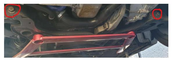
Loosen both front control arm bolts leave the left bolt sticking out about 2cm as shown below and fully remove the other side.
