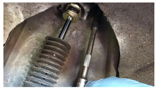
Then replace the bolt you removed with a washer and bolt supplied with the strut bar. Then remove the 2<sup>nd</sup> bolt which you left in and replace with a new bolts and washer. then repeat the process for the other side of the car.
