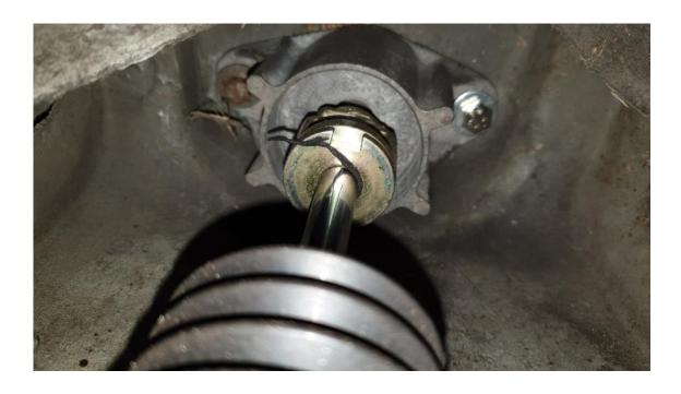
As you can see the new bolts are longer which allows you to put the strut bar on top then shock bolts. You can now take put the car back down on the ground.
